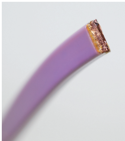
Fig. 1. PEEK magnet wire insulations are becoming increasingly popular in the high-voltage range. They are very resistant and can withstand high temperatures and voltages. This ensures higher reliability compared to the use of enameled wires. © Solvay
